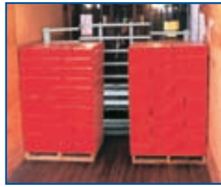
Spread loads against the inside trailer walls.
