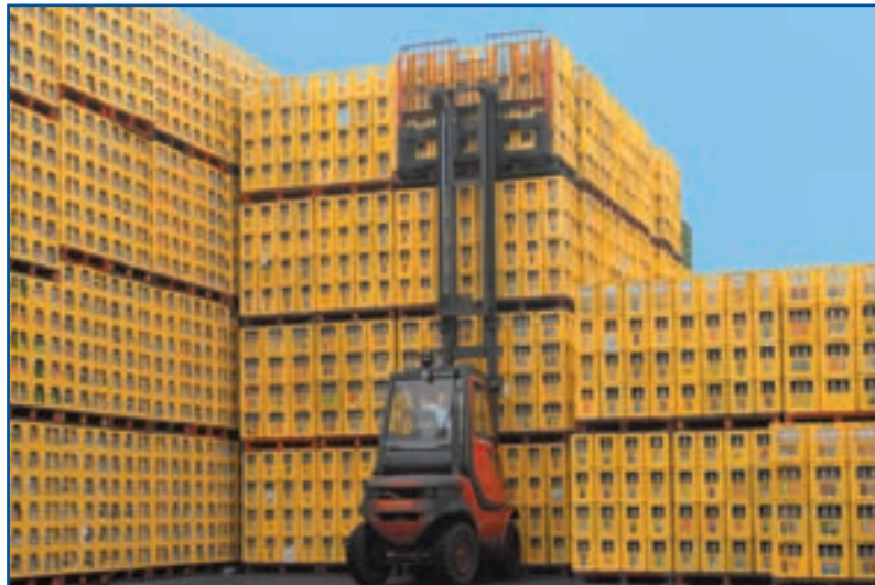
Narrow frame allows same maneuverability as a single-load truck.
